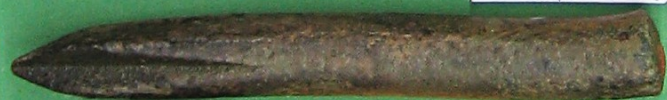
COPPER-ALLOY SPIKE -PROBABLY THE END OF A WW2 ARMY RADIO EARTHING ROD. BROAD ARROW ON IT. 371 C 15-5-97
