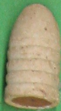
0.55" MINIÉ BALL FOR AN ENFIELD 3-BAND RIFLE OF 1859. UNFIRED. BASE PLUG OF CLAY & WAX. C SEVEN ACRES 906 1102F 2.2.99
