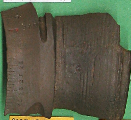
PART OF AN ANTI- AIRCRAFT SHELL TIMING RING. STILE PARK 977 1493C 4-6-99
