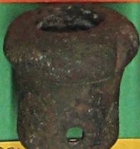
BRASS HORN PROTECTOR. WITH COARSE TAPERED THREAD, TWO NOTCHES & RETAINING PIN HOLE
